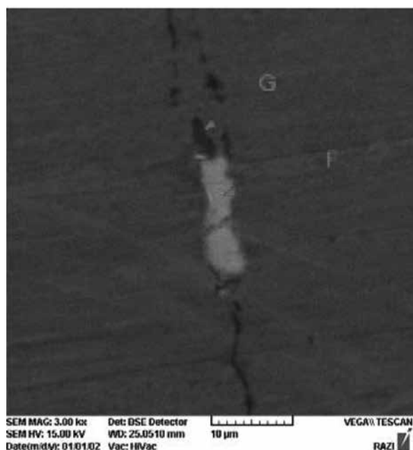
Figures 32.4. Back-scattered electron image of sound metal and inclusions (by the authors, 2011).
